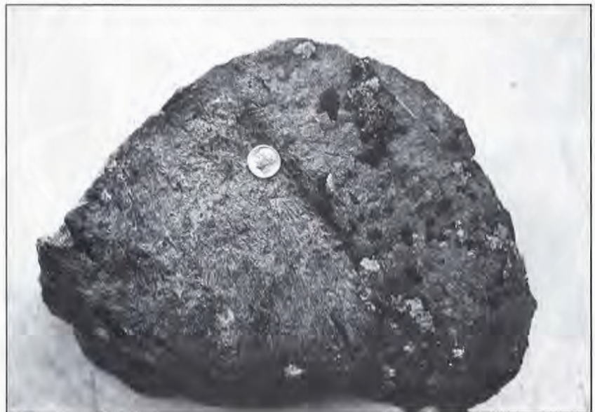
Figure 10. Random spinifex texture in a tremolite schist from the Sunday Morning Creek area of the Seminoe Mountains. (Photograph by W.D. Hausel, 1989.)
