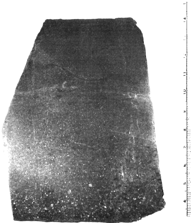
A TYPICAL GRADED SUBGRAYWACKE BED (BC-45) FROM MINERAL FORK IN THE BIG COTTONWOOD CANYON AREA
